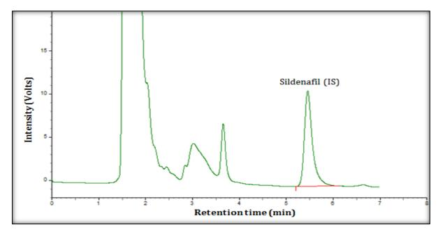
**Figure 3.16** A processed zero serum sample spiked with sildenafil; the internal standard of propranolol analysis.
